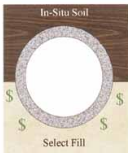
Type 1 Installation – Money is in the Backfill
