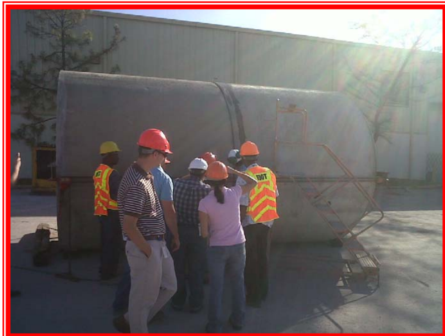
FDOT engineers inspect a hydrostatic joint test on 96-inch RCP at Rinker's Miami pipe plant on December 21, 2011.
